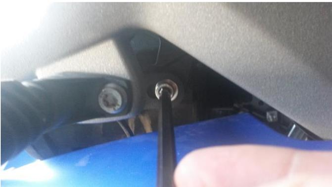
**Step 3:** The arm is positioned correctly if the rivet nut is extruding towards the headlight.
