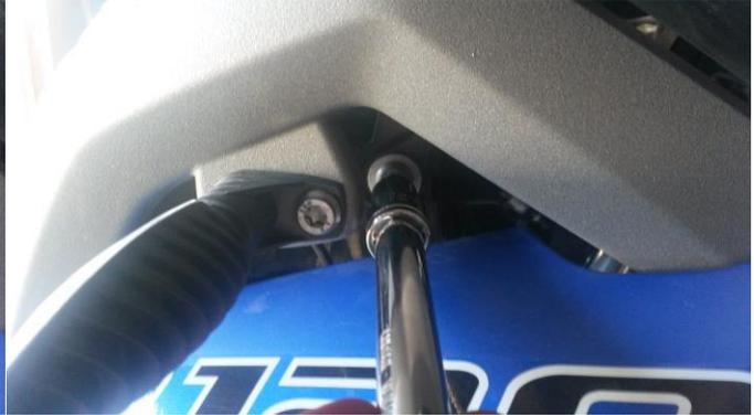
**Step 2:** Take one M6 bolt and washer supplied and one side arm. Position the arm and insert the bolt and tighten it loosely.
